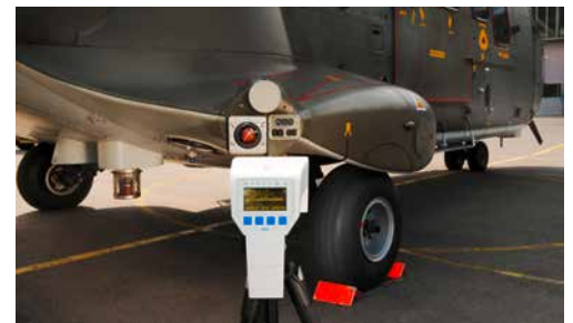
Testing a helicopter's EW system with missim
