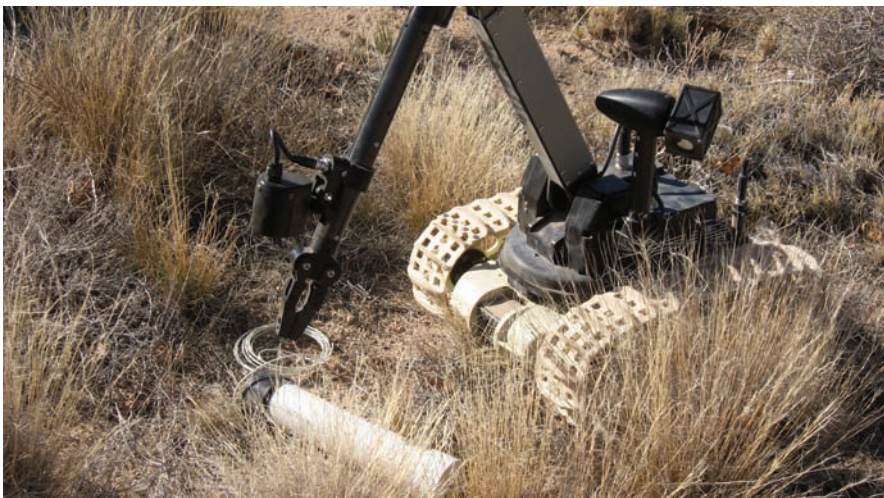
Dragon Runner 20 SUGV can be carried in a standard-issue pack, and can lift from 5 to 10 lbs with its manipulator arm.
